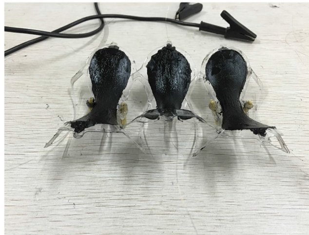
Figure 17. 3-segment annelid robot.
