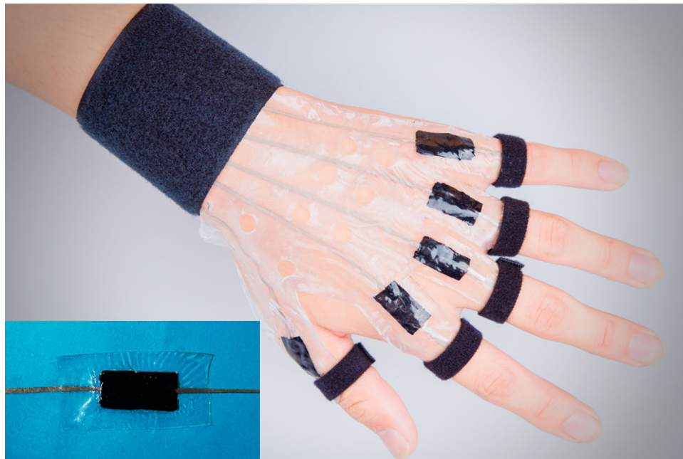
Figure 2. (a) Structure of a single sensor; (b) SkinGest prototype for gesture recognition.
