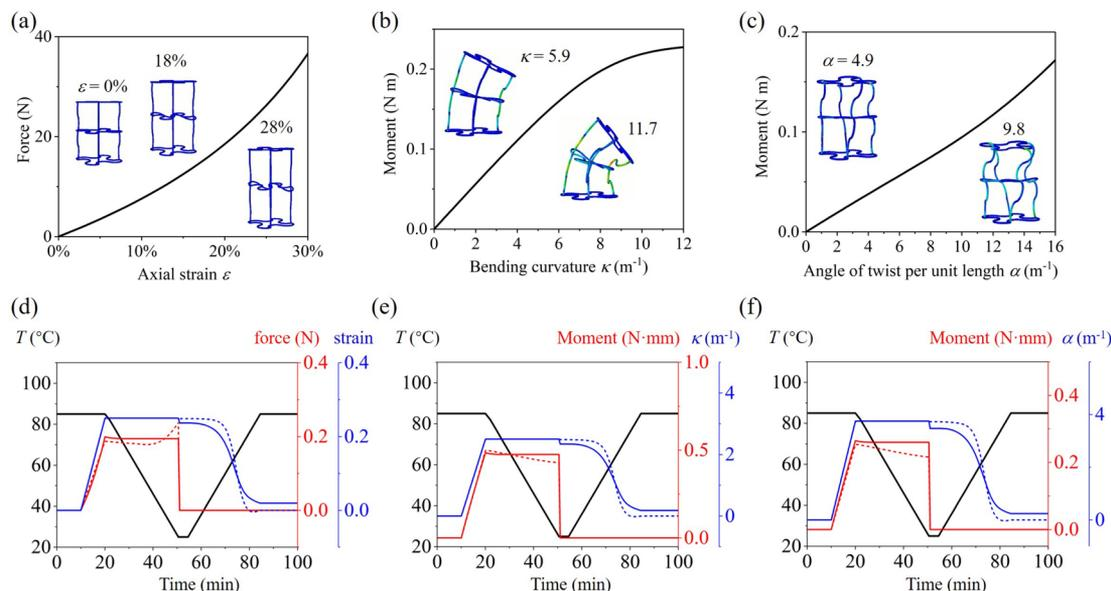
**Figure 6.** Shape memory behaviors of a  $1 \times 1 \times 2$  3D horseshoe lattice. (a–c) Loading–displacement curves of the lattice structure under axial, bending, and twisting loadings at room temperature, respectively. Insets show the deformed shapes at different strains. (d–f) Theoretical (dashed curves) and FE simulated (solid curves) shape memory behaviors of the 3D horseshoe structure programmed by axial, bending, and twisting loadings in strain control mode, respectively.
