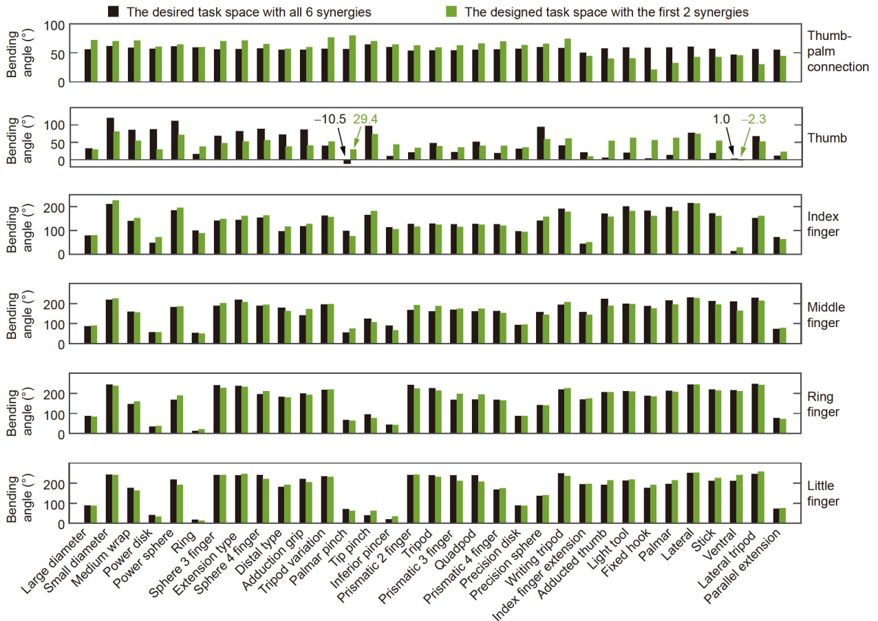
Figure 9 (Color online) Comparison of desired task space (with all 6 synergies) and designed task space (with the first 2 synergies) on actuator bending angles.
