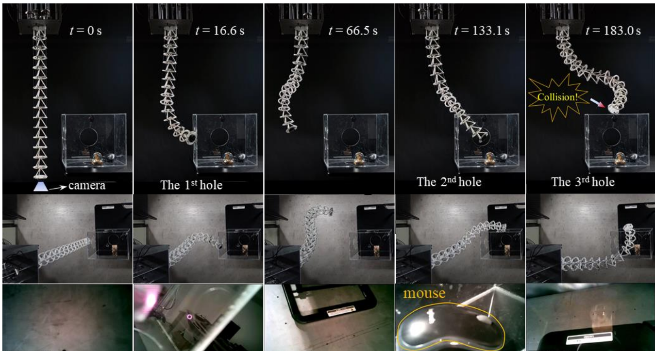
Fig. 22 Experimental snapshots for Strategy 1 from the main view, the top view and the camera at the TCR's end.
