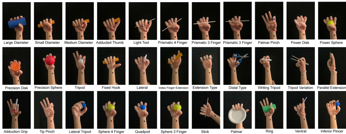
Fig. 5. The Feix GRASP taxonomy carried out by the proposed hand. Our hand can achieve all the 33 grasps in the GRASP taxonomy. Here, the dyed soft hand is adopted for the experiment.
